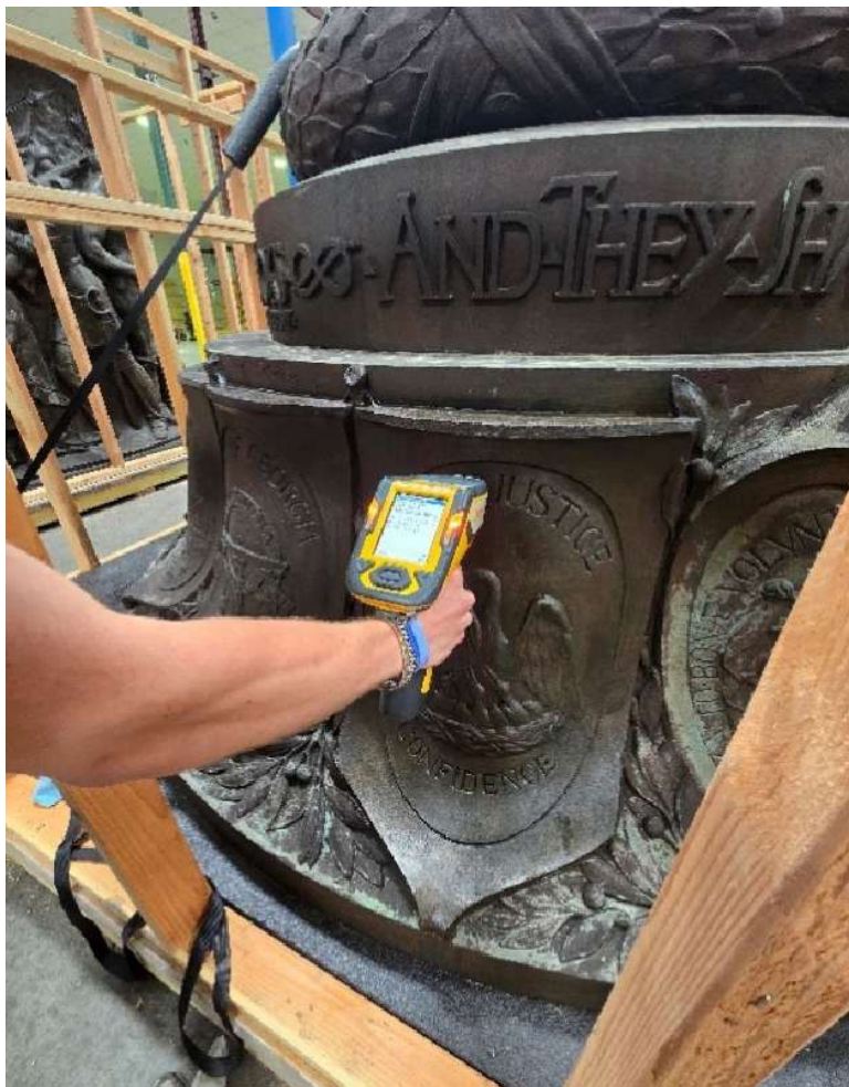
Testing bronze composition with handheld X-ray fluorescence (XRF) analyzer
