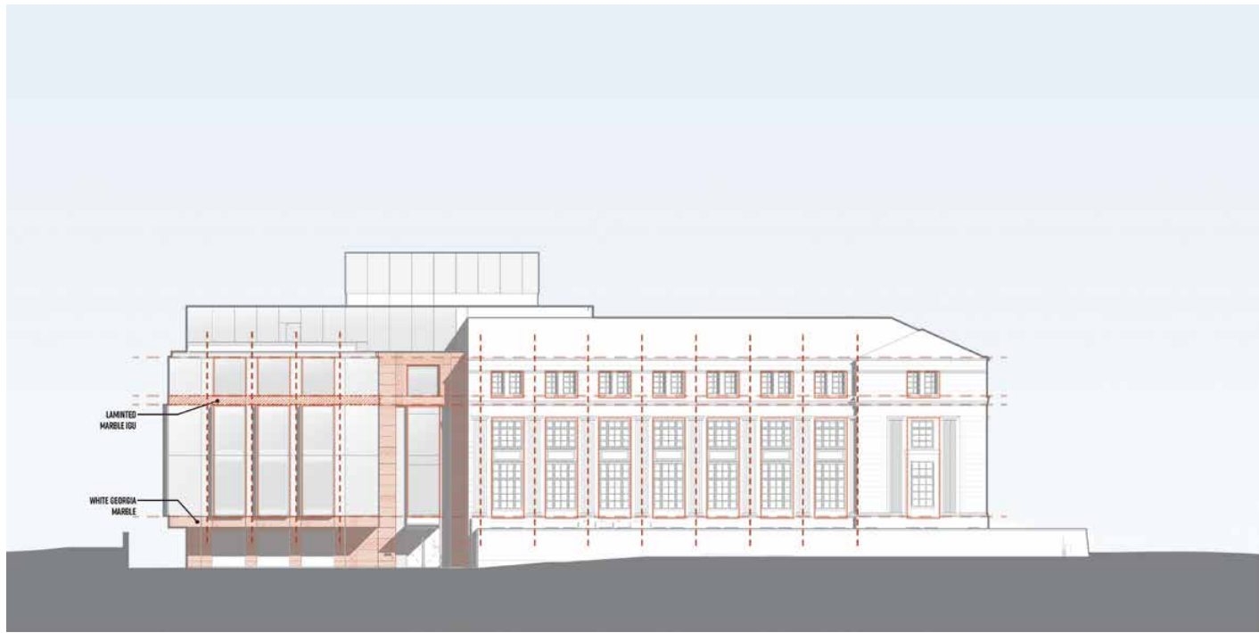
Tying new addition into FRB-East Building through the use of white Georgian marble
