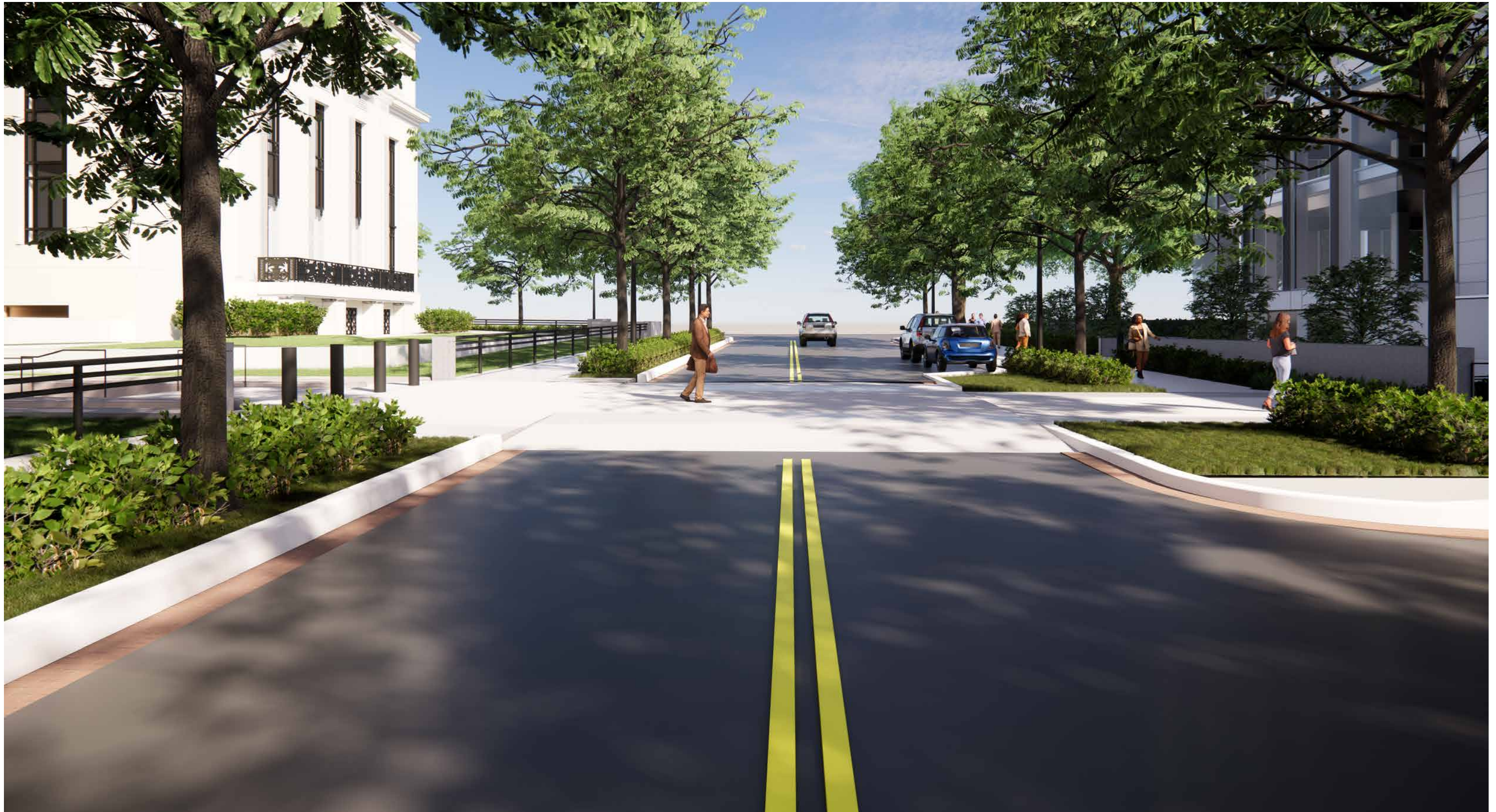
32'-6" WIDE - PARKING LANE BULB-OUT AT CROSSWALK
