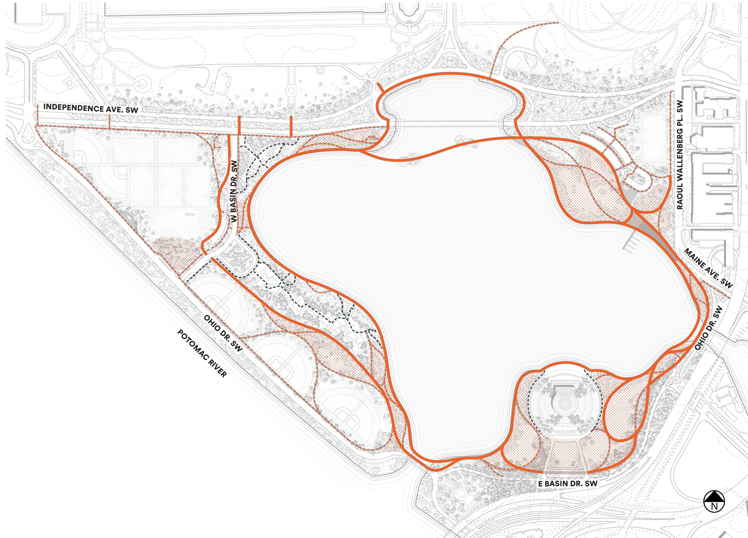
Diagram showing differentiation of 12 ft wide versus 6 ft – 8 ft wide pathways across site and existing pathways to remain. All pathways are accessible. Open circulation shows zones of free pedestrian movement.
