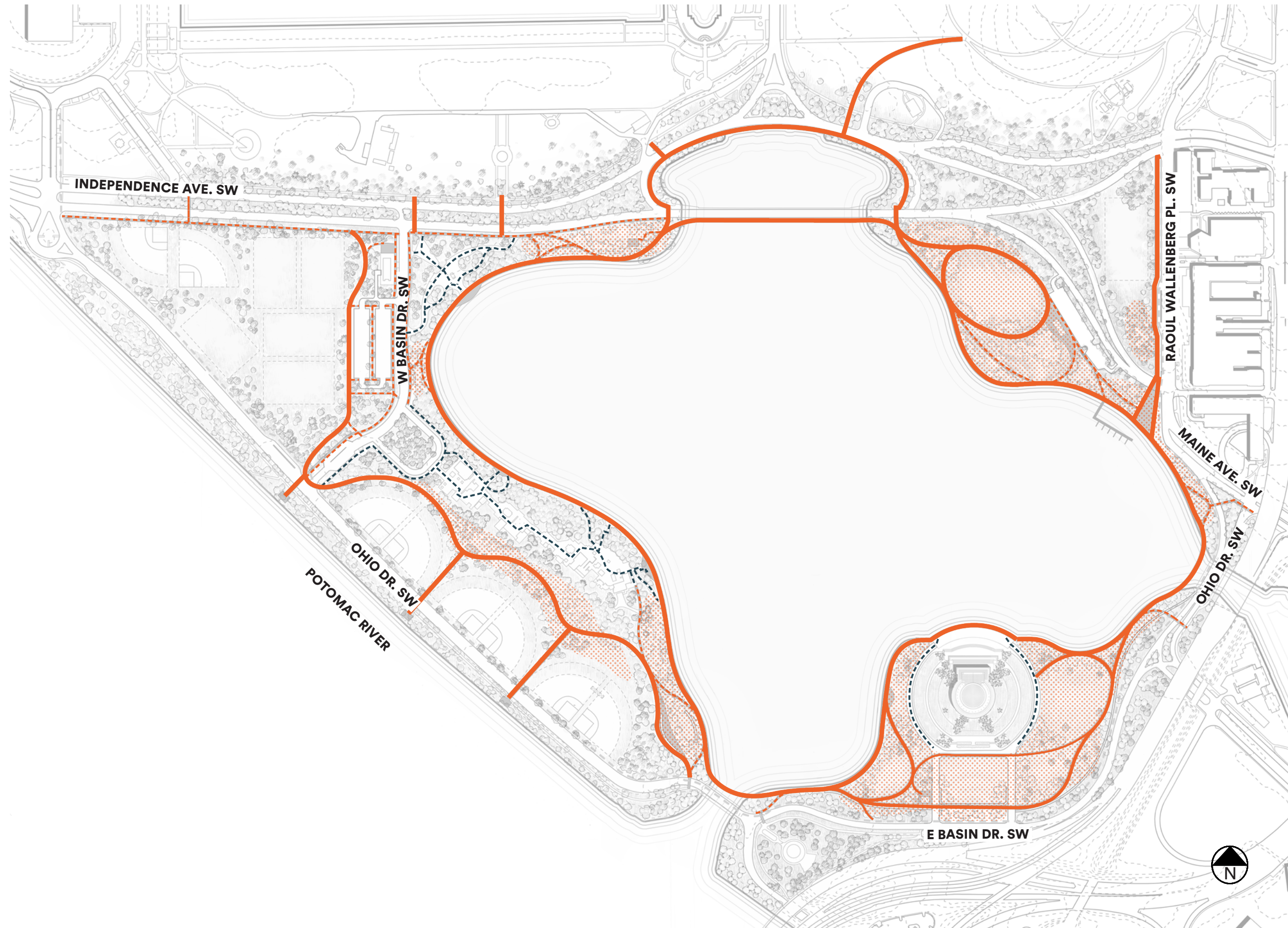
Diagram showing differentiation of 12 ft wide versus 6 ft – 8 ft wide pathways across the site and existing to remain walkways. All pathways are accessible. Open circulation shows zones of free pedestrian movement.
