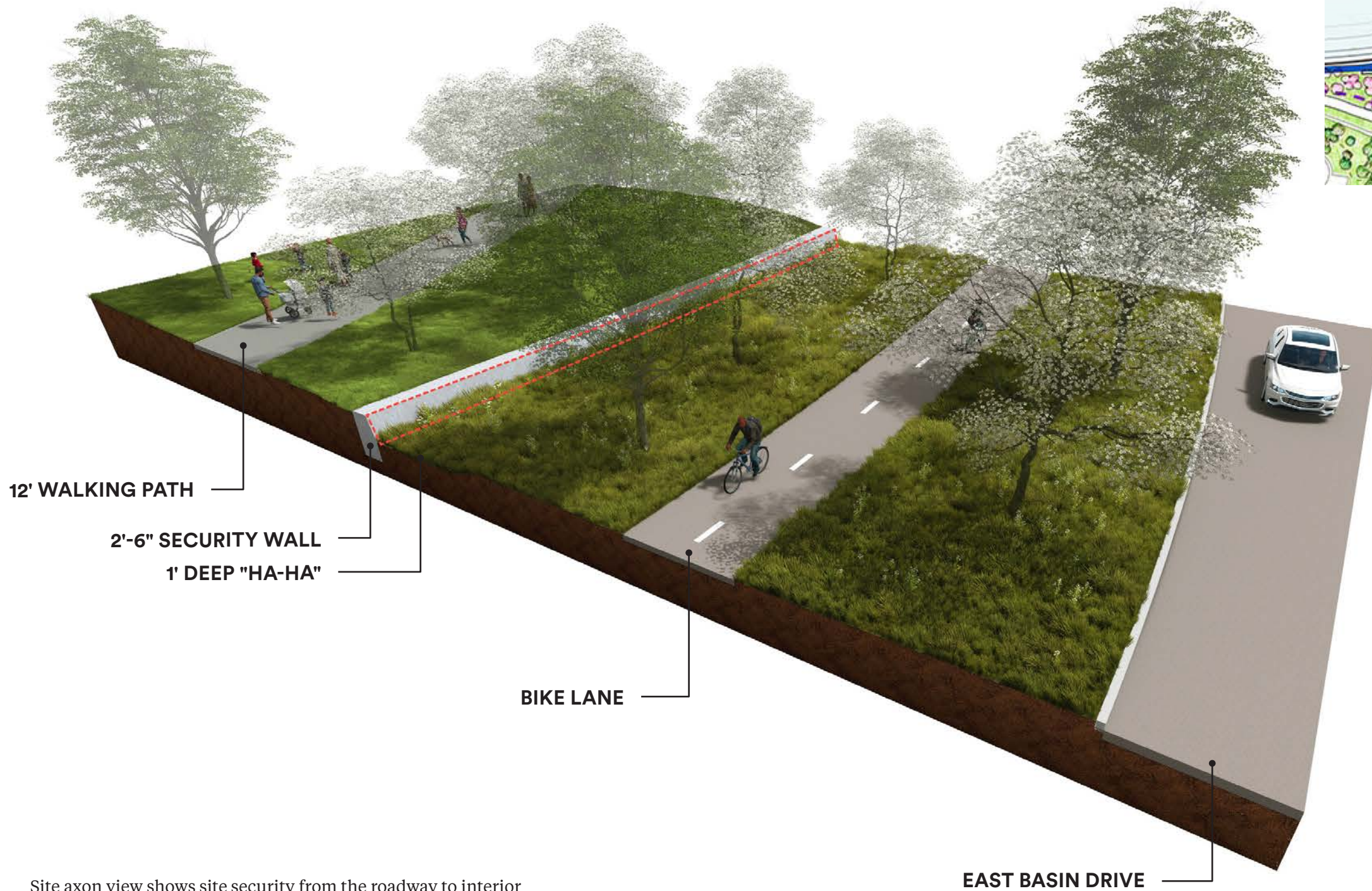
Site axon view shows site security from the roadway to interior pedestrian pathways. Secure edge highlighted in red dashed line.
