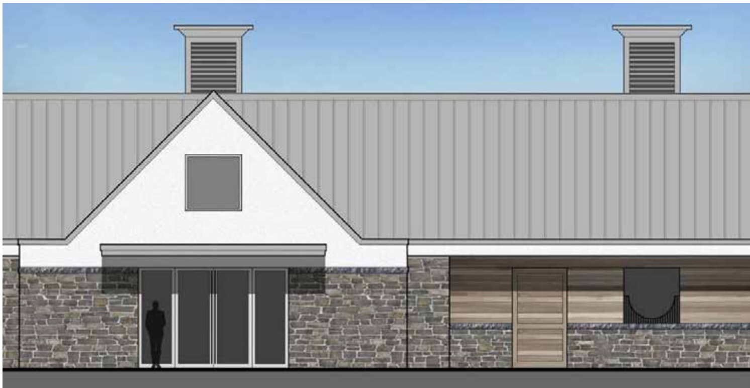
TEAK WOOD SIDING OVER SEMI-COURSED GRANITE FIELDSTONE MIX WITH MORTARED JOINTS AND SPLIT-FACE GRANITE COPING
