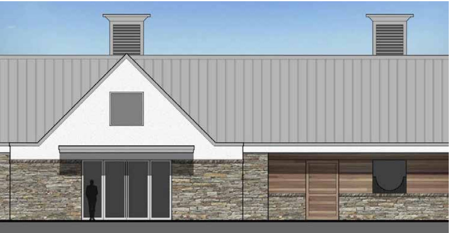
MAHOGANY WOOD SIDING OVER SEMI-COURSED VARIEGATED GRANITE WITH TIGHT JOINTS AND SPLIT-FACE LIMESTONE COPING
