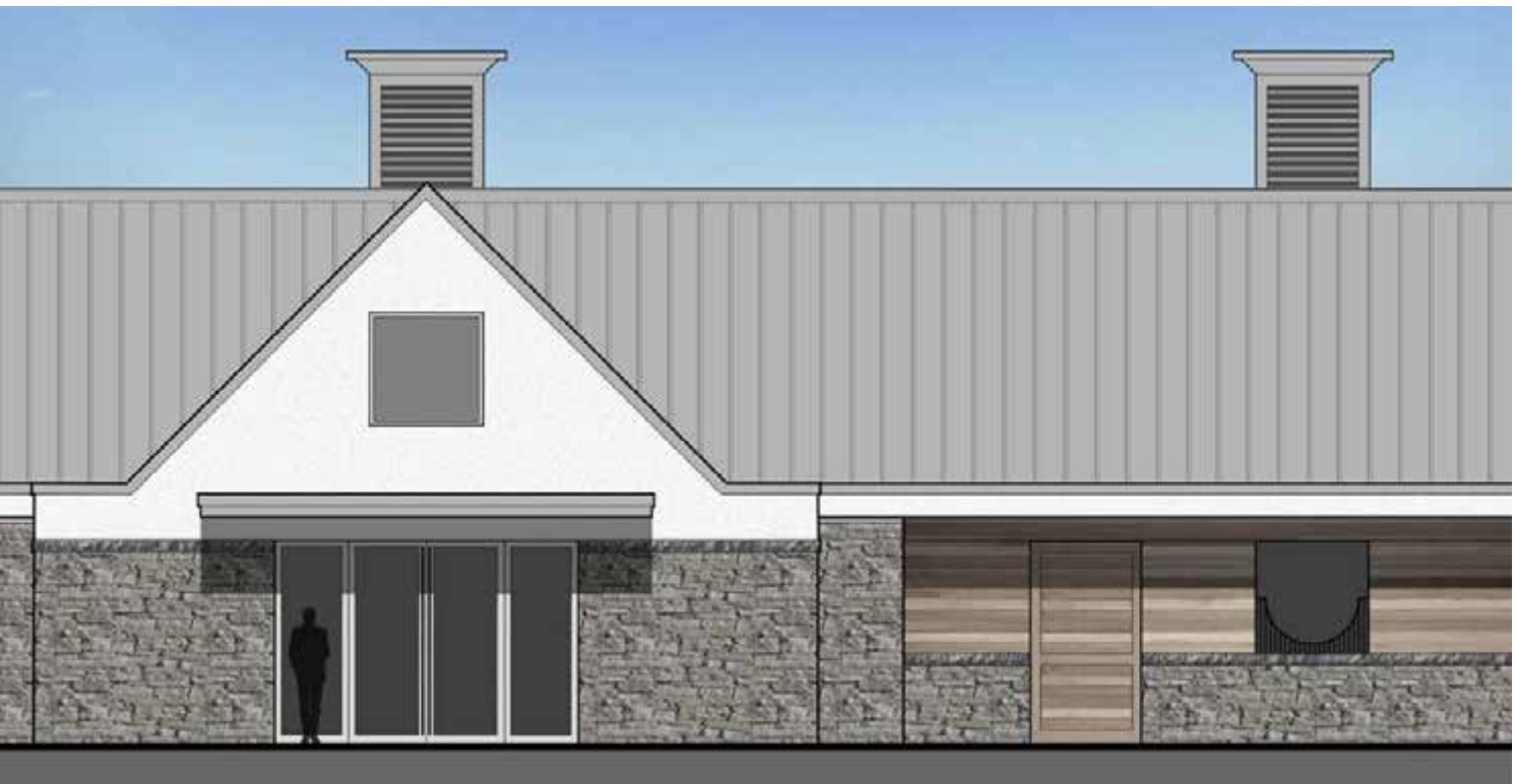
HIGH PERFORMANCE MODIFIED WOOD SIDING (COLOR TBD) OVER SEMI-COURSED GREY GRANITE MIX WITH TIGHT JOINTS AND SPLIT-FACE GRANITE COPING
