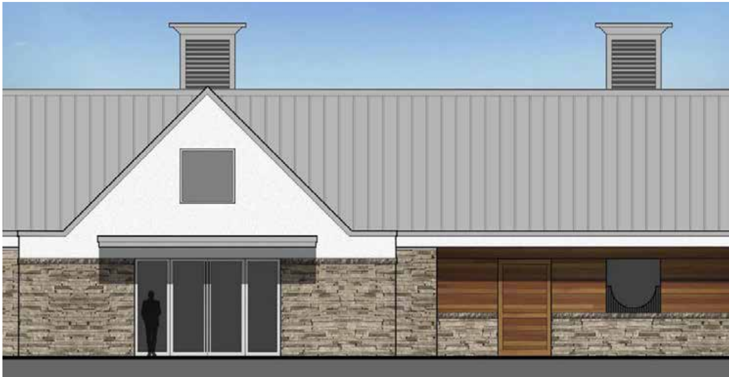
IPE WOOD SIDING OVER SEMI-COURSED LIMESTONE MIX WITH TIGHT JOINTS AND SPLIT-FACE LIMESTONE COPING
