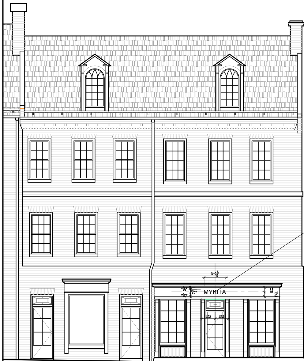
1 A001 DEMOLITION M STREET (SOUTH) ELEVATION 1/4" = 1'-0"
