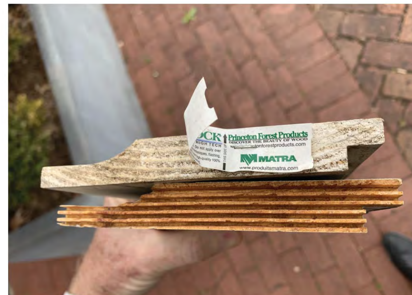
EXISTING PINE SIDING BY PRIMELOCK - 5" EXPOSURE, FINGER JOINTED
