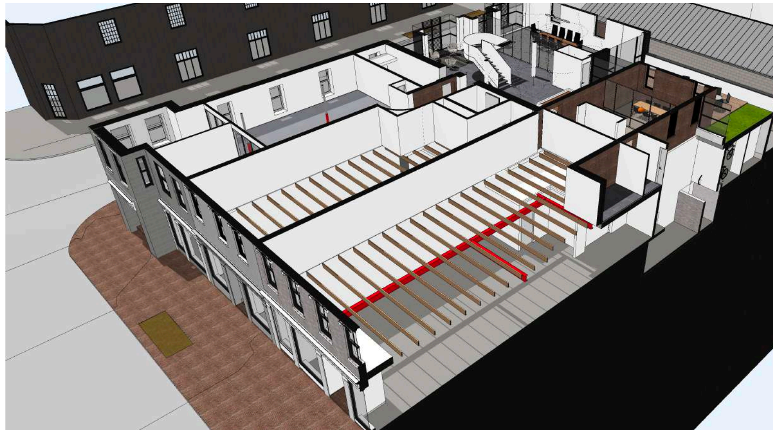
Retail space cutaway showing remaining existing structure
