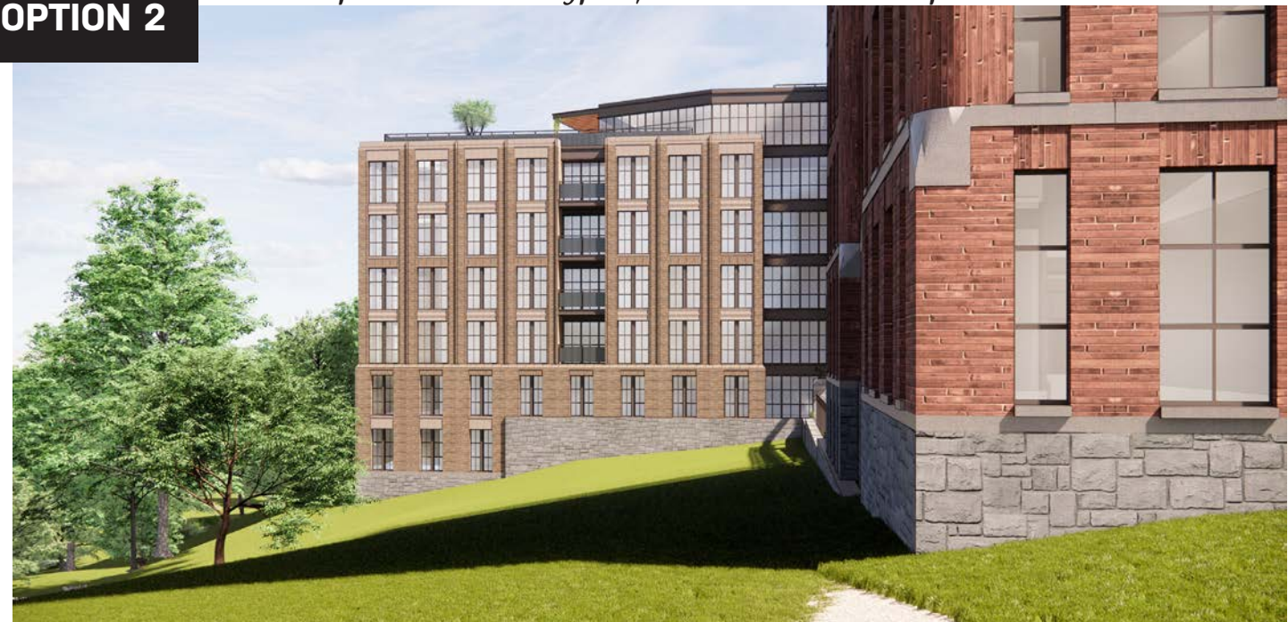
New roof line & window type w/ cast-stone sills and spandrels
