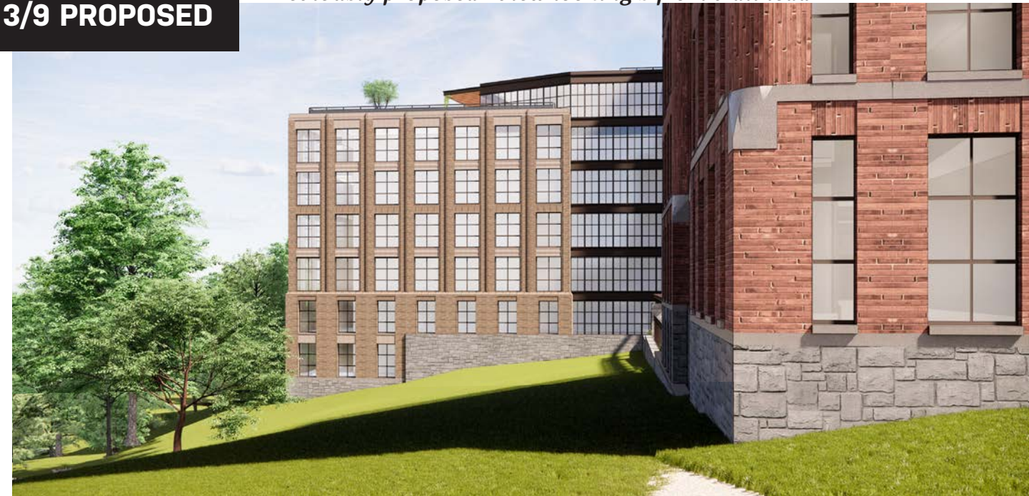
New window type w/ single-level articulation of cast stone lintels and sills
