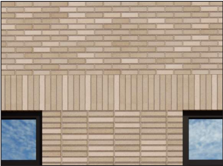
C: Stacked Brick Details Base Windows
