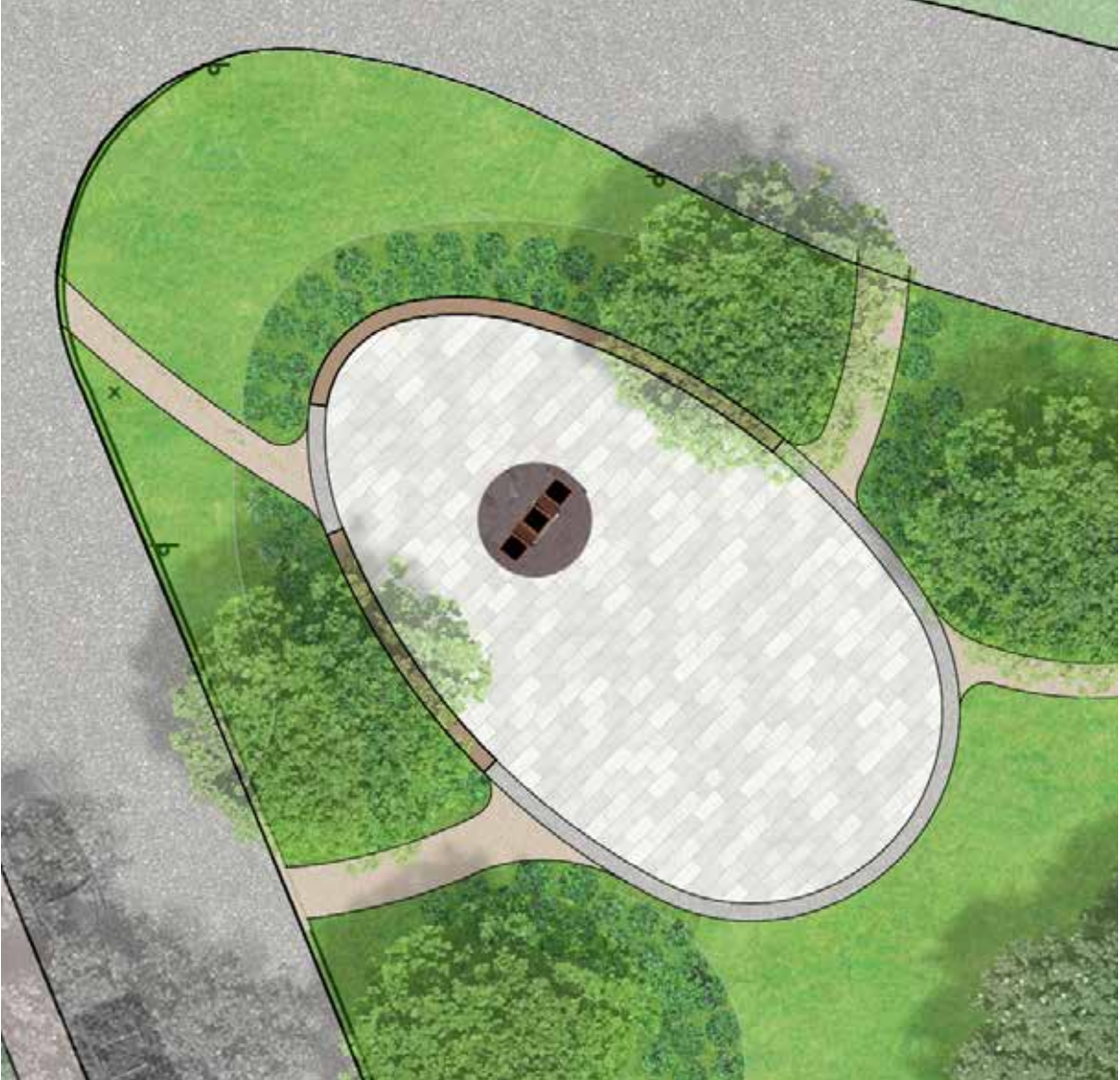
PLAN DETAIL - WTC STEEL ARTIFACT (E-0017) POLISHED CUT MARBLE PLINTH W/ INTEGRATED LIGHTING - 316 SST STRUCTURAL SUPPORT FITTINGS
