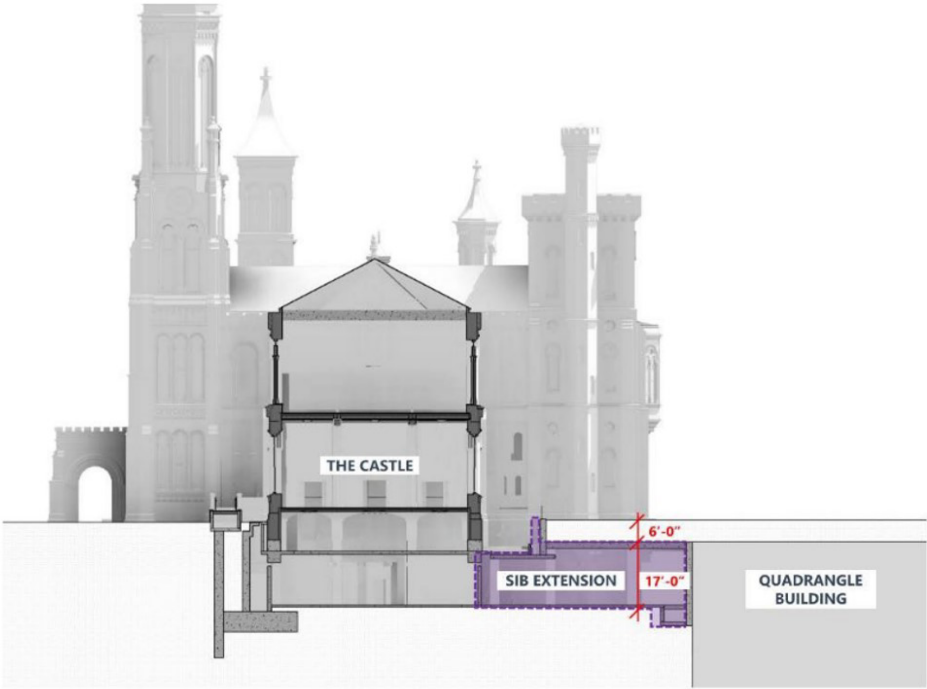
Figure 3.3.2.b – SIB Extension building section
