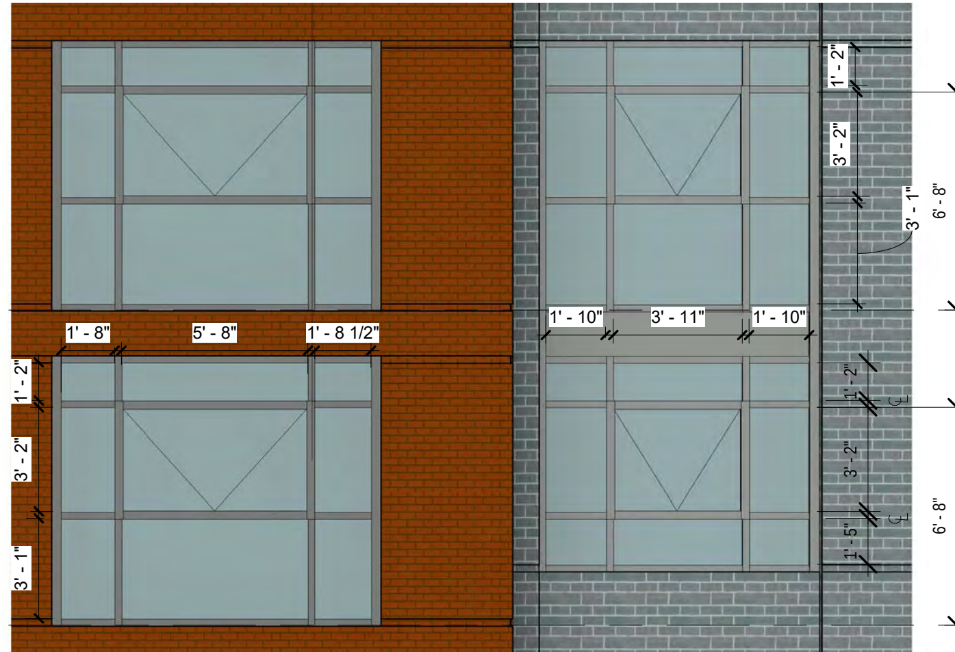
NEW WINDOWS IN RED BRICK
