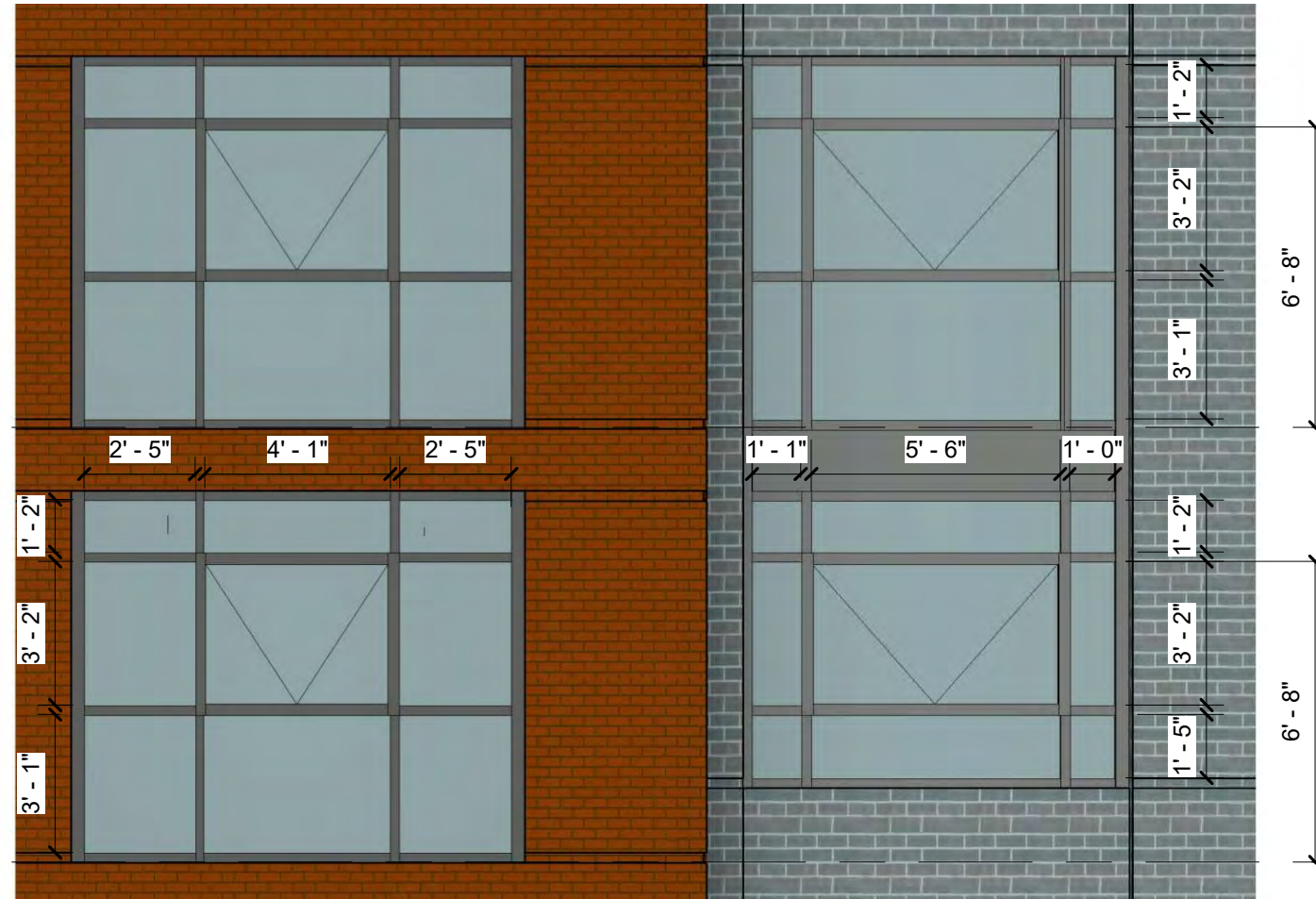
NEW WINDOWS IN RED BRICK
