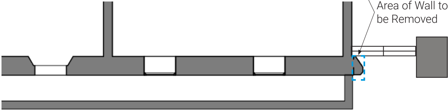
UNMODIFIED UNFINISHED END-WALL CONDITION OVERLAPPING NEW CONSTRUCTION
