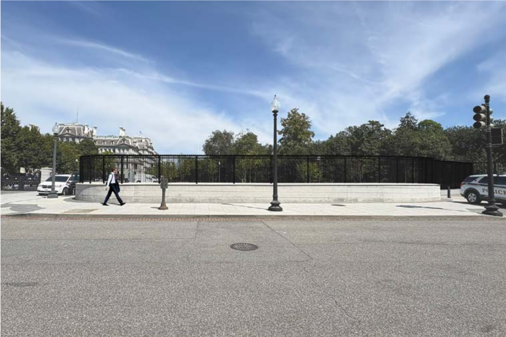
PROPOSED VIEW LOOKING NORTH AT RETAINING WALL FROM E STREET SHOWING TEMPORARY 6-FOOT-TALL DECORATIVE METAL FENCE ABOVE EXISTING GRANITE RETAINING WALL AND SUPPORTED BY BALLASTS BEYOND (NOT VISIBLE FROM THIS PERSPECTIVE).
