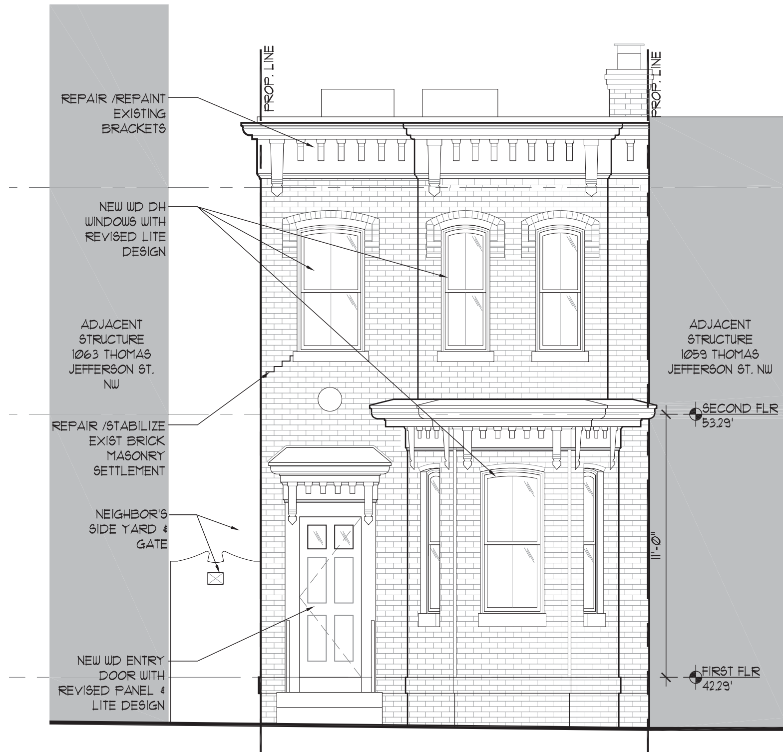
1 PROPOSED WEST ELEVATION SCALE: 1/4" = 1'-0"
