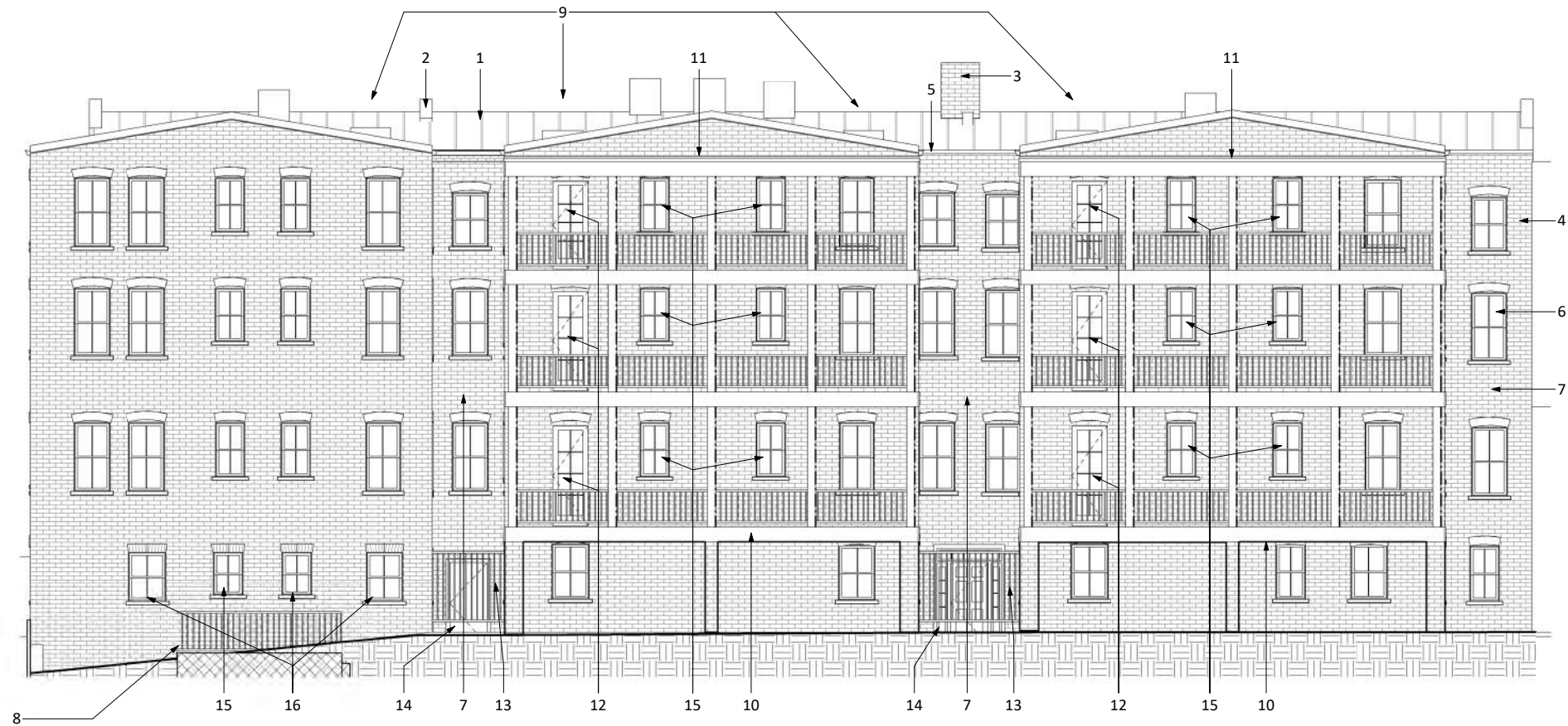
1 | PROPOSED REAR ELEVATION P-203 | 3/16" = 1'-0"
