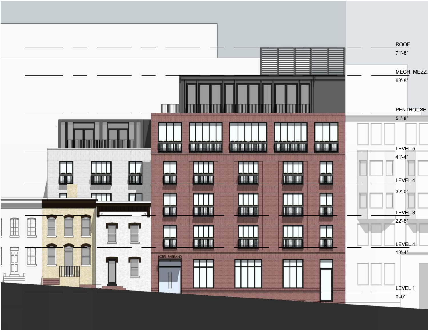
PREVIOUS DESIGN ELEVATIONS DO NOT MATCH EXISTING CONDITION AFTER FIELD VERIFICATION PREVIOUS DESIGN IS 3'-5" HIGHER THAN NEW PROPOSED DESIGN
