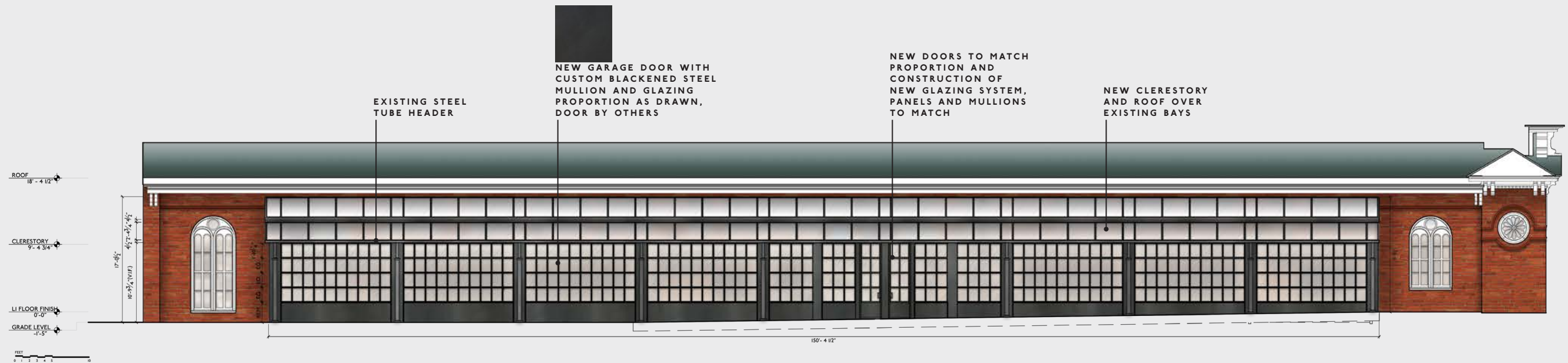
2 SOLARIUM ELEVATION - PROPOSED SCALE: 1/8" = 1'-0"
