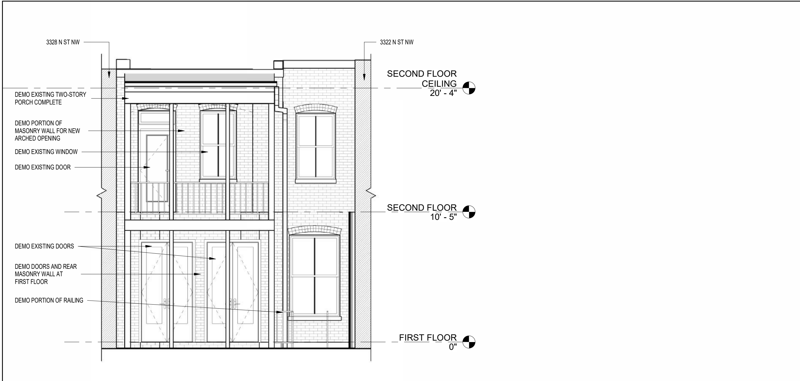
1 EXISTING REAR ELEVATION 1/4" = 1'-0"
