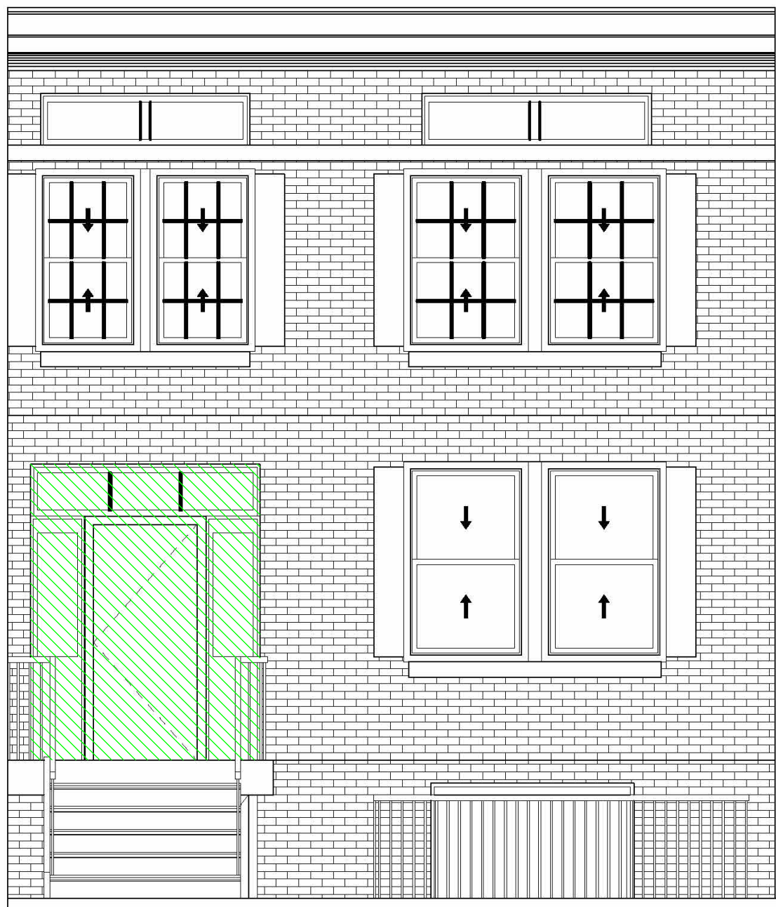
FRONT DOOR REPLACEMENT
