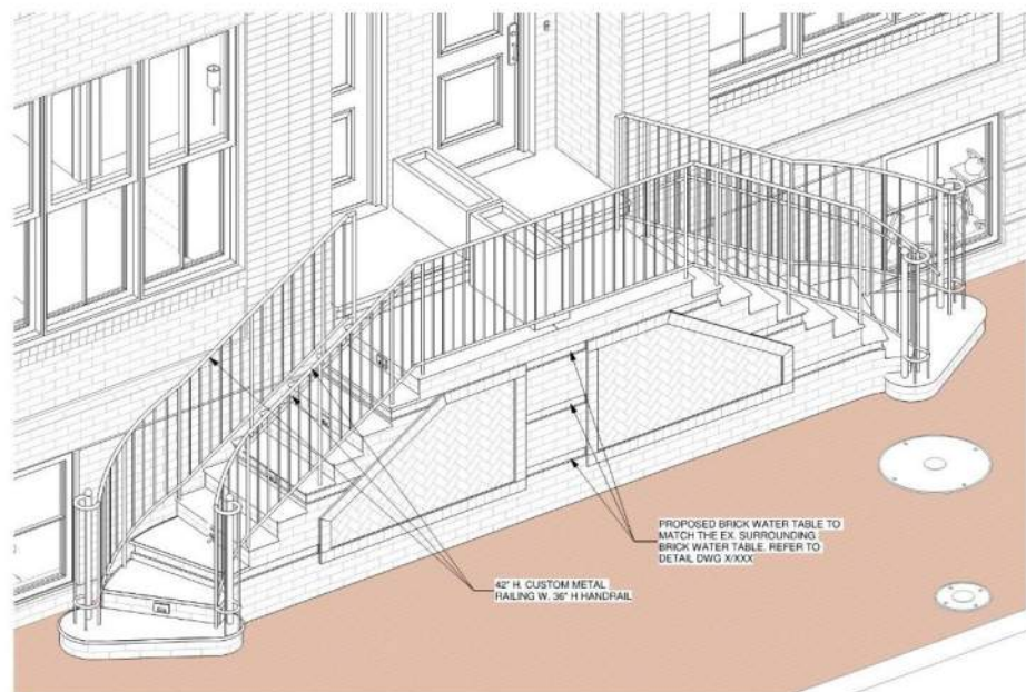
3 UNIT 2 & 3 - ENTRY STAIRCASE 3D VIEW SCALE:
